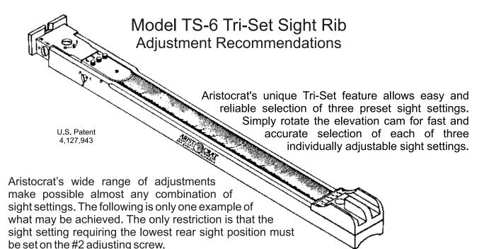
Sighting in is accomplished as follows: First turn the slotted elevation screw all the way to the bottom. Then rotate it back up one half to one full turn. This screw is not used again except to compensate for lighting or ammunition variables.
